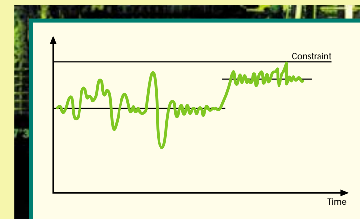
FIGURE 2: SQUEEZING THE VARIANCE ALLOWS MOVING THE MEAN VALUE CLOSER TO THE CONSTRAINT.
